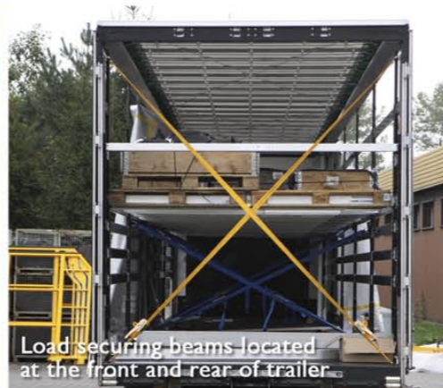
Perforated side beams allow for flexible location of supports for different loads
