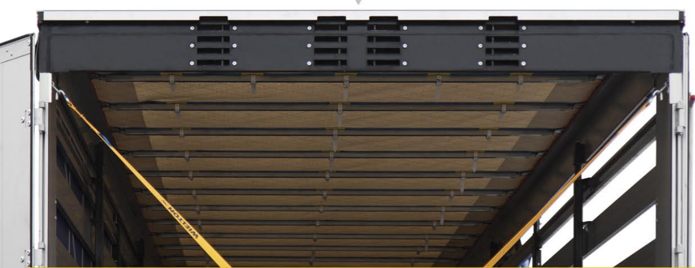
Construction giving possibility to set up inner height on four different levels.
