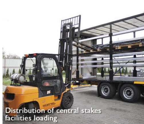
Construction of central stakes allows for loading of goods at various heights
