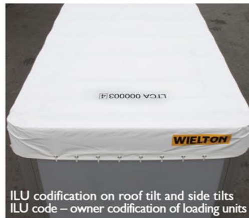
24 double lock buckles on each side
