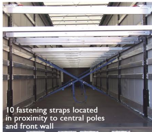
Second level flooring with maximum load bearing of 900kg fitted with 22 loading beams
