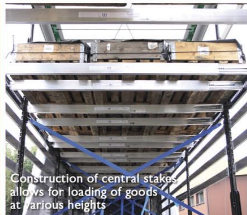
Load securing beams located at the front and rear of trailer
