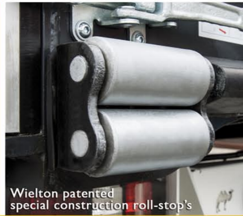
Rubber bumping blocks on rear end skirt protecting door locks
