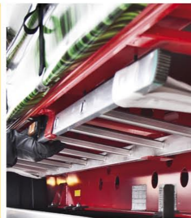
Self-locking ladder mounting (on side)
